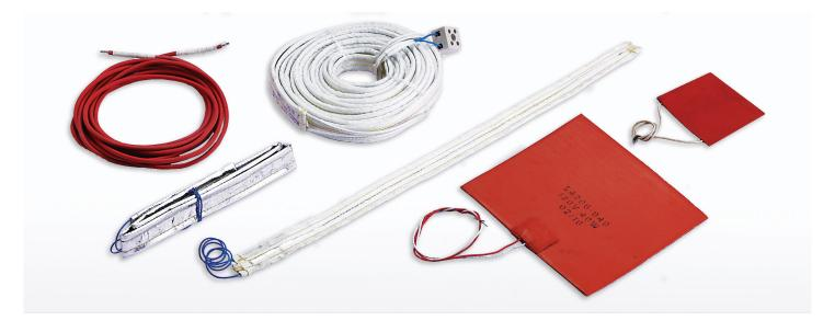
Helical heating coil insulated with fibre glass sleeve & tape suitable for maximum 100 Deg. C. skin temperature. It will have terminal leads with ceramic connector at either end.
